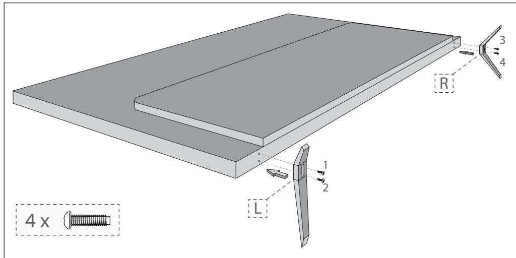
**English:** To assemble the base stand to the TV you will need a cross head screwdriver. To avoid damage to the TV screen during assembly ensure the TV is placed on a soft flat surface with the LCD screen facing downwards.
